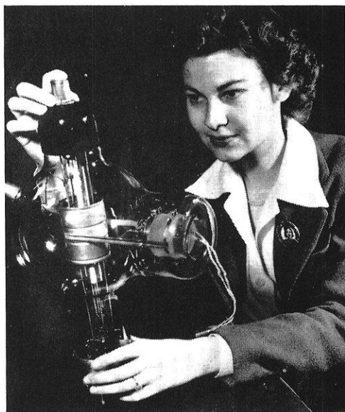
PLASTICS HAVE MANY USES —Use of the ceramic plastic, "Prestite," as bases for high frequency radio tubes manufactured by Heintz and Kaufman, Ltd., South San Francisco, California, side stepped possible material shortage. Prestite combines the electrical and mechanical strength of wet process porcelain with the moulding qualities of dry process porcelain. It is used in many products where intricate shapes must meet high insulation requirements.
