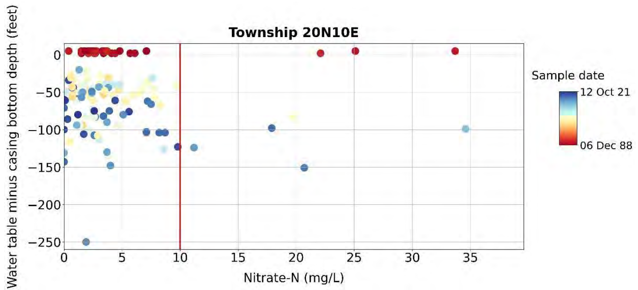
Figure C 73. Township 20N10E. (top) Yearly average nitrate concentration versus year of sampling. Dashed line indicated linear regression of the data. R^2 is the goodness of fit of the linear relationship. (bottom) Nitrate concentration versus the difference between the static water table and the casing depth. Color refers to the sampling date: the oldest measurements are marked with a red color, the most recent measurements are marked with a blue color.
