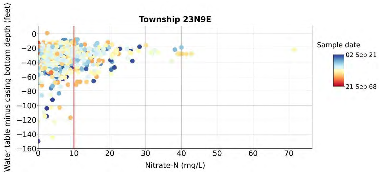
Figure C 101. Township 23N9E. (top) Yearly average nitrate concentration versus year of sampling. Dashed line indicated linear regression of the data. R^2 is the goodness of fit of the linear relationship. (bottom) Nitrate concentration versus the difference between the static water table and the casing depth. Color refers to the sampling date: the oldest measurements are marked with a red color, the most recent measurements are marked with a blue color.
