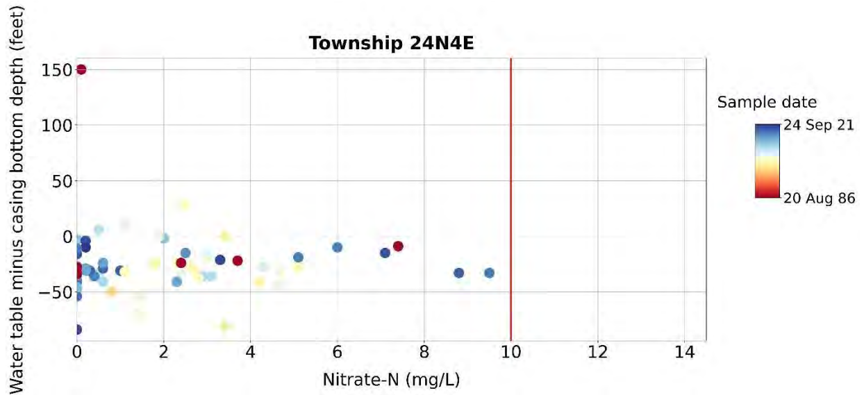
Figure C 105. Township 24N4E. (top) Yearly average nitrate concentration versus year of sampling. Dashed line indicated linear regression of the data. R^2 is the goodness of fit of the linear relationship. (bottom) Nitrate concentration versus the difference between the static water table and the casing depth. Color refers to the sampling date: the oldest measurements are marked with a red color, the most recent measurements are marked with a blue color.
