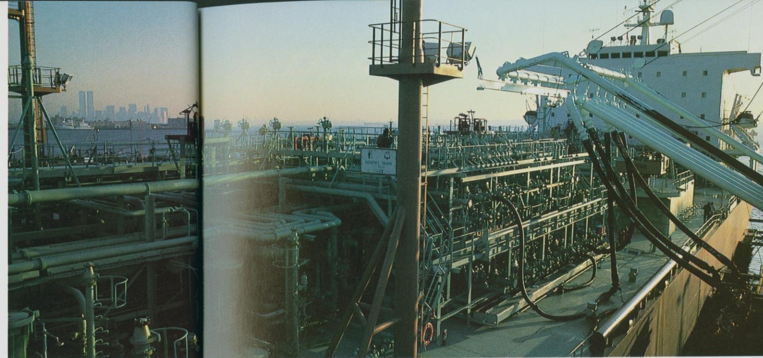
The Exxon Wilmington is one of two 42,000 dwt specialty tankers commissioned by the company in 1984 to replace older, less efficient vessels in U.S. specialty service. Capable of carrying 43 different products in separate cargo tanks, the ship is shown unloading petroleum products at the Bayonne, New Jersey, terminal, which was modernized to accommodate the new vessels.
