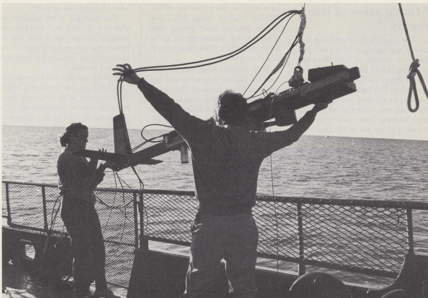
The electronic "fish" is hoisted aboard the Neeskay . The "fish" transmits sounds and records echoes used to census fish populations.
