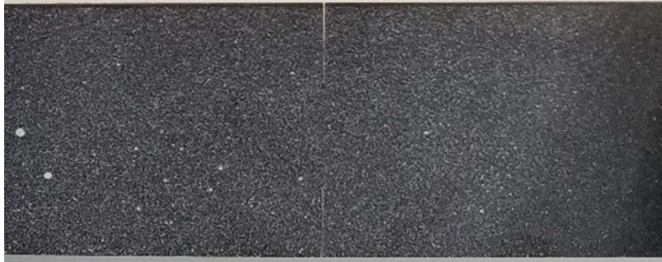
Figure 9-6: DEC-plate with applied speckle pattern
