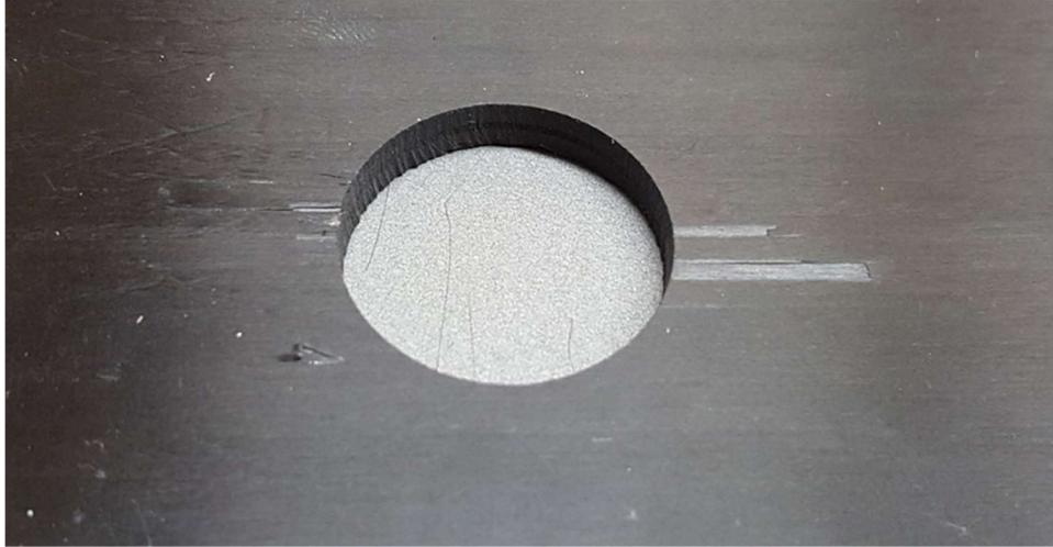
Figure B-3: Flaking in the composite laminate when directly drilling into the coupon to create a start-up hole
