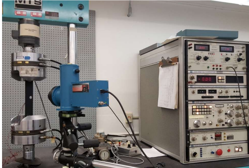
Figure 6-2: TSA experimental set-up
