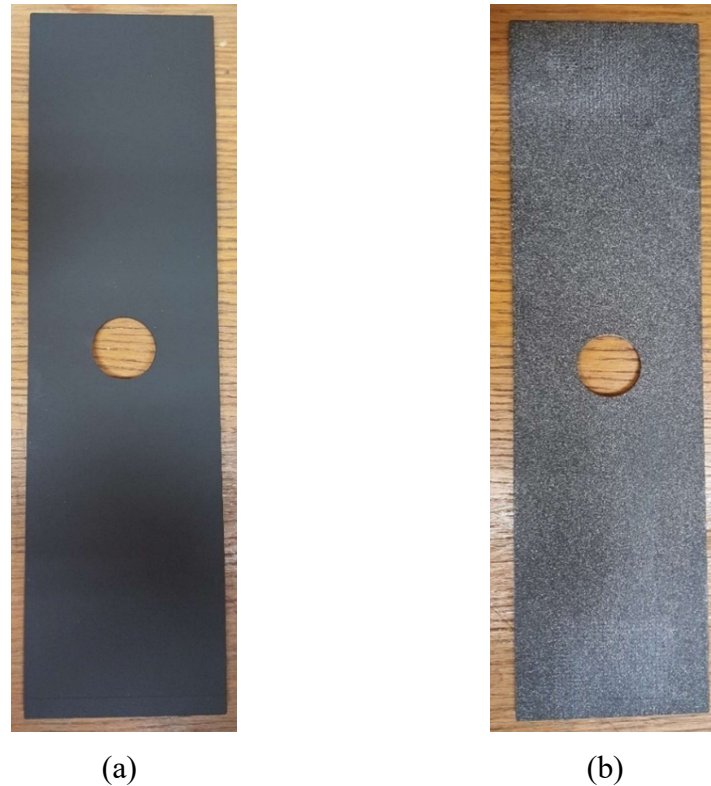
Figure 4-3: (a) Plate covered with a thin layer of black paint and (b) Speckle pattern on the plate
