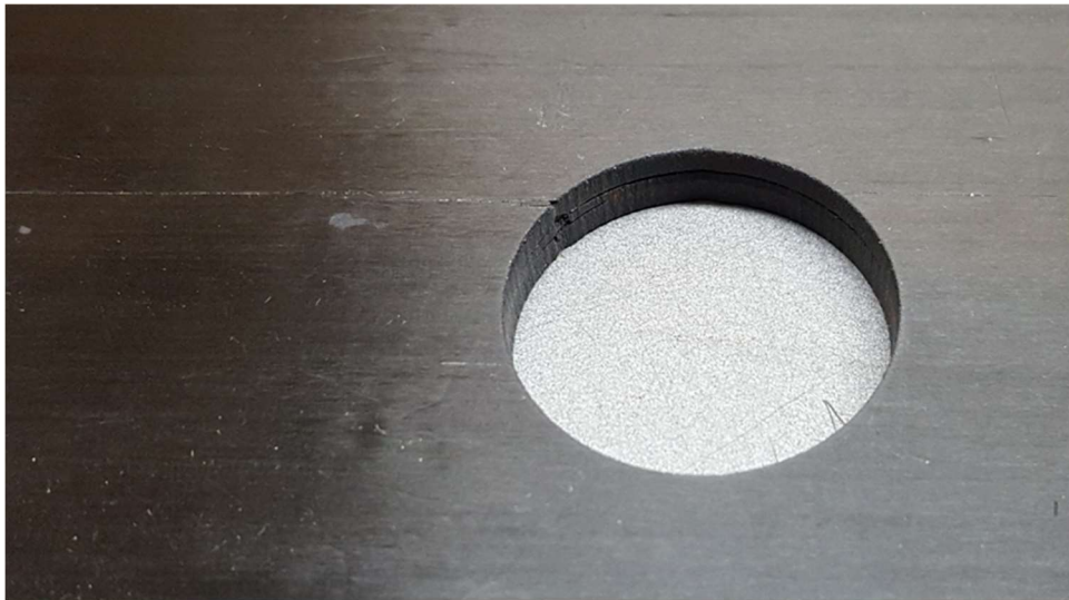
Figure B-2: Delamination in the composite laminate when using a stainless-steel plate on top of the composite coupon when creating a circular hole using water-jet cutting
