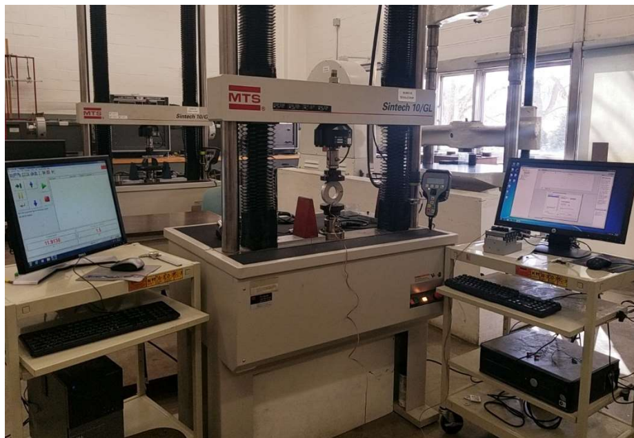
Figure 7-13: Loading and strain data acquisition of strain-gage mounted aluminum ring
