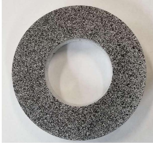
Figure 7-3: Aluminum ring with applied speckle pattern
