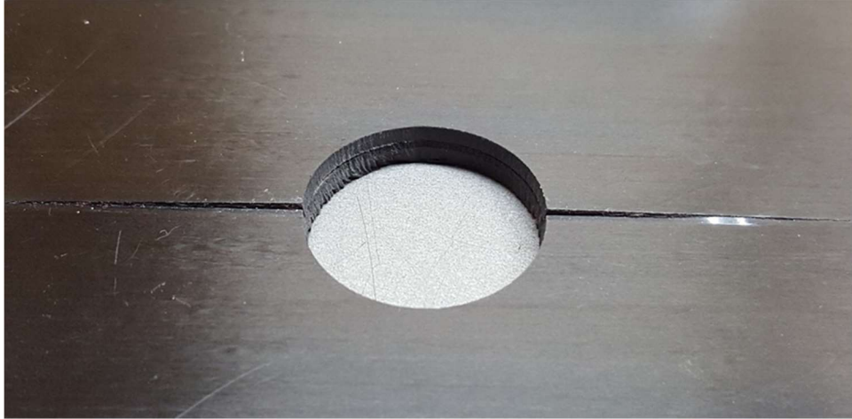
Figure B-1: Severe delamination in the composite laminate due to creating a circular hole directly using water-jet cutting
