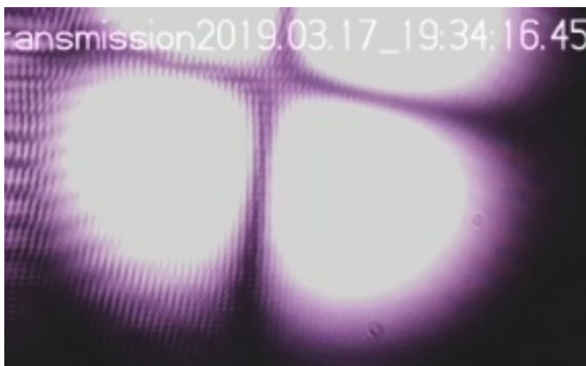
Figure 2.10: ULE cavity transmission taken by a Raspberry-Pi camera. The laser is locked to a stable mode of the cavity.
