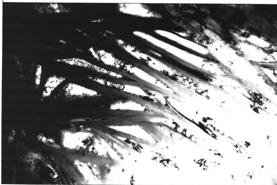
Color-enhanced transmission electron micrograph of melt-spun Nd 0.4 Fe 0.6 having 7.5 kOe coercivity.
