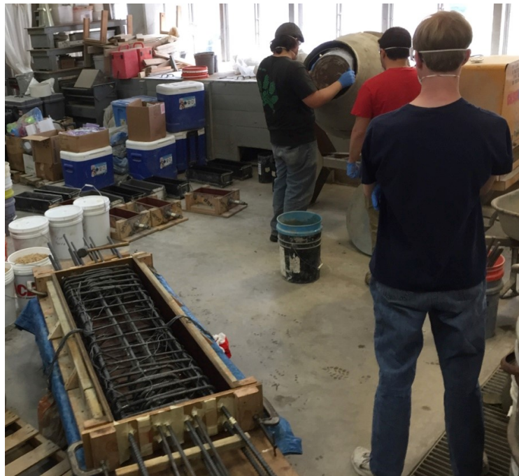
Figure 3.8: Mixing SFRC and Coupling Beam Specimen Ready for Casting.
