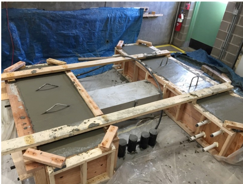
Figure 3.11: Finished Coupling Beam Specimen.
