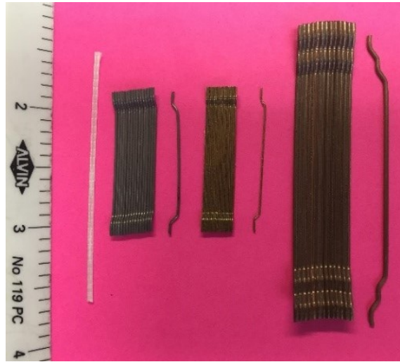
Figure 2.1: Examples of Fibers used to Reinforce Concretes (scale: inches).
