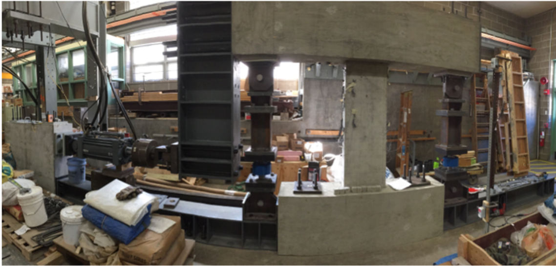
Figure 3.12: Coupling Beam Test Setup.
