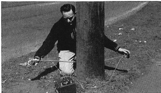
3. Transistorized circuitry was designed. And a Sonic Pole Tester was built and tested.
