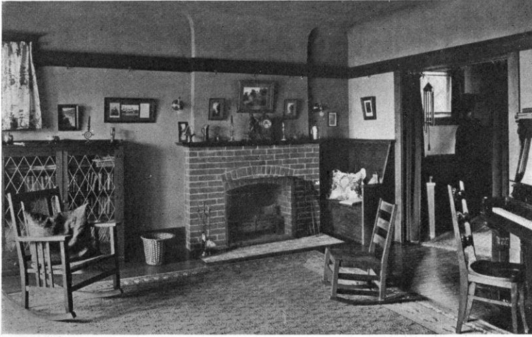
AN INVITING CORNER OF THE LIVING ROOM: THE FIRESIDE SEAT SERVES AS A WOOD-BOX, AND THE BASKET-GRATE BURNS EITHER WOOD OR COAL.
