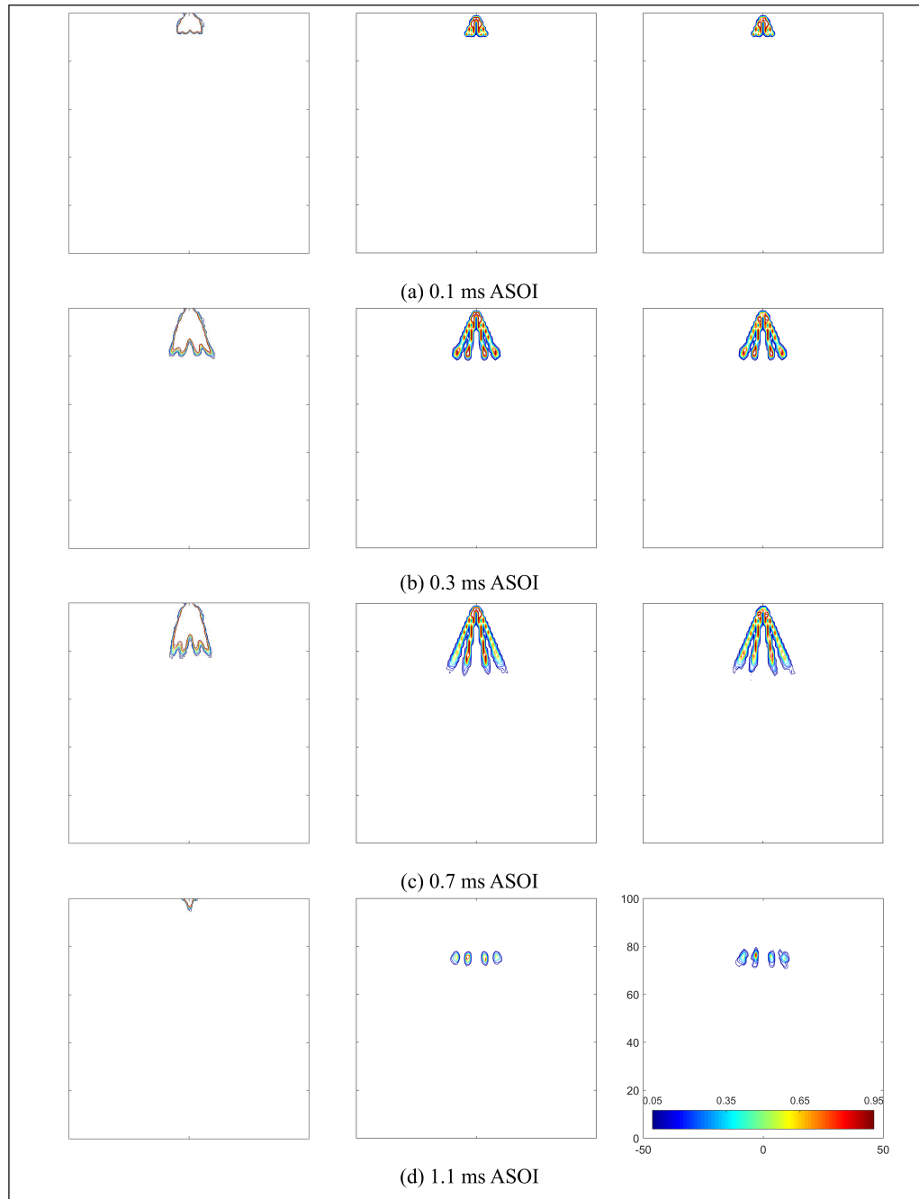
Figure 5.28: Liquid probability contours for case 3 at various times from experiments (left column), LHS (middle column), and PCE (right column). For each contour, there is a 95% chance of producing a liquid region that has the same size as indicated by the innermost region, and a 5% chance of producing a liquid region that has the same size as indicated by the outermost region.
