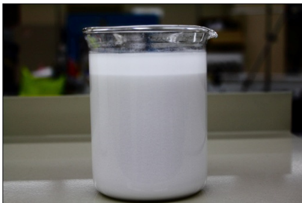
Figure 2-3: \text{Al}_2\text{O}_3 suspension immediately after the ultrasonic treatment
