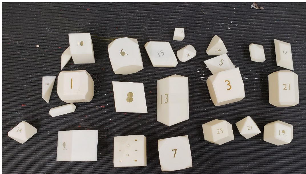
Figure 4. The 3D printed versions of the blocks. These were printed using ivory color. The 3D printing files have since been modified to fix inhomogeneity in block size.
