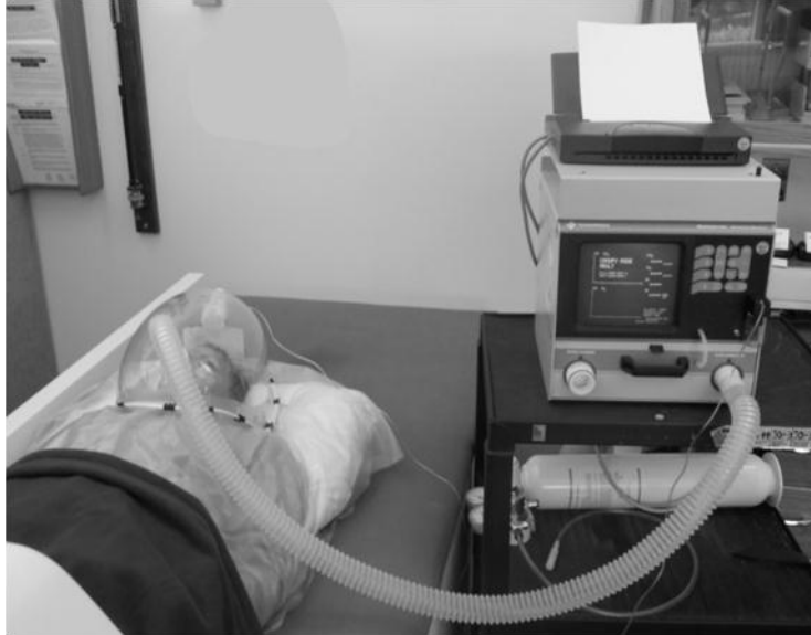
Figure 1: The Deltatrac (DTC) metabolic cart indirect calorimeter system in-use. During testing, subjects were instructed to remain motionless without sleeping while respiratory gases were drawn from a clear hood canopy placed over the participant's entire head, as shown. The final 20 minutes were used to calculate respiratory exchange ratio (RER; VCO_2 \div VO_2 ), as well as RMR (kcal/day) using the modified Weir equation (17): [3.941 \times VO_2] + [1.106 \times VCO_2]
