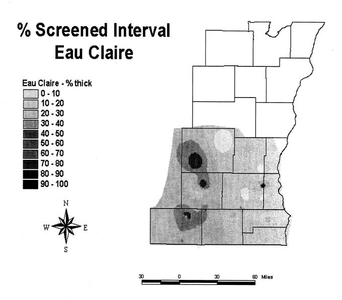
**Figure 7:** Percent of the screened interval of wells in the Cambro-Ordovician aquifer of eastern Wisconsin that is open to the Eau Claire Formation. The Eau Claire Formation is defined only in the southern half of the study area.
