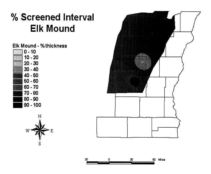
**Figure 5:** Percent of the screened interval of wells in the Cambro-Ordovician aquifer of eastern Wisconsin that is open to the Elk Mound Formation. The Elk Mound Formation is defined only in the northern half of the study area.
