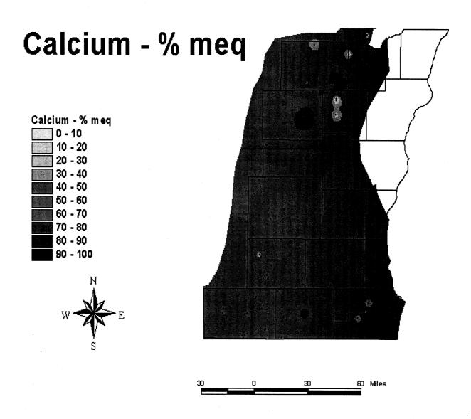
**Figure 15:** The percent of total cations in water produced from wells in the Cambro-Ordovician aquifer of eastern Wisconsin that is attributable to calcium. Expressed as % milliequivalents. Black spots indicate individual wells.
