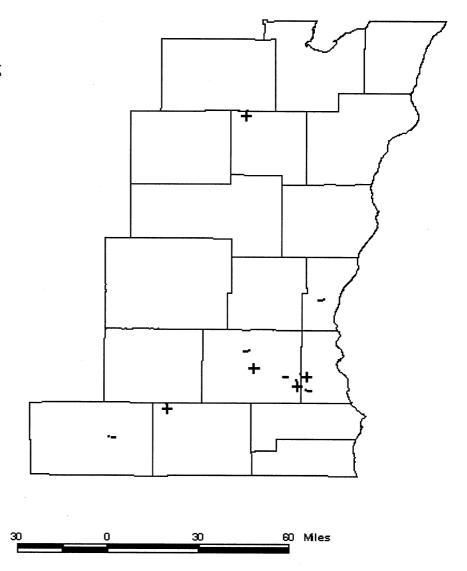
**Figure 12:** Location of wells that exhibit a salinity rate of change. Wells that exhibit a decrease in salinity greater than 10 ppm/year are indicated by - . Wells that exhibit an increase in salinity greater than 10 ppm/year are indicated by + .
