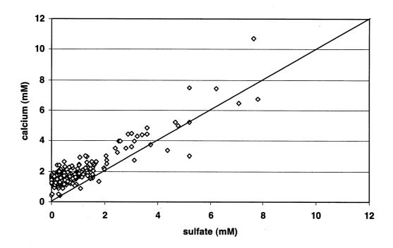
**Figure 13:** Molar relationship between calcium and sulfate in Cambro-Ordovician wells of eastern Wisconsin. Line indicates the 1:1 molar ratio.
