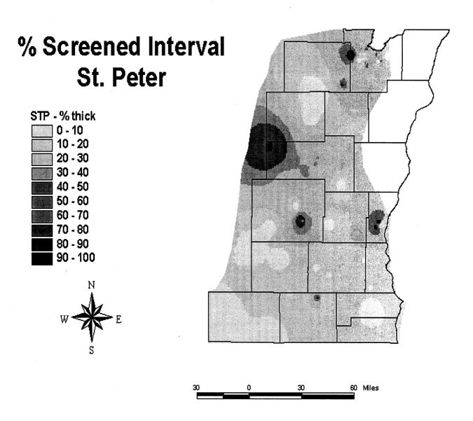
Figure 3: Percent of the screened interval of wells in the Cambro-Ordovician aquifer of eastern Wisconsin that is open to the St Peter Formation Formation.
