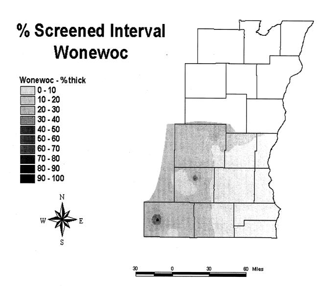
**Figure 6:** Percent of the screened interval of wells in the Cambro-Ordovician aquifer of eastern Wisconsin that is open to the Wonewoc Formation. The Wonewoc Formation is defined only in the southern half of the study area.
