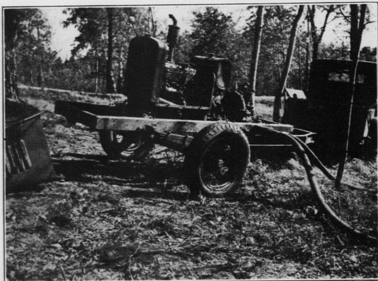
Trailer pumping unit built by conservation department.
