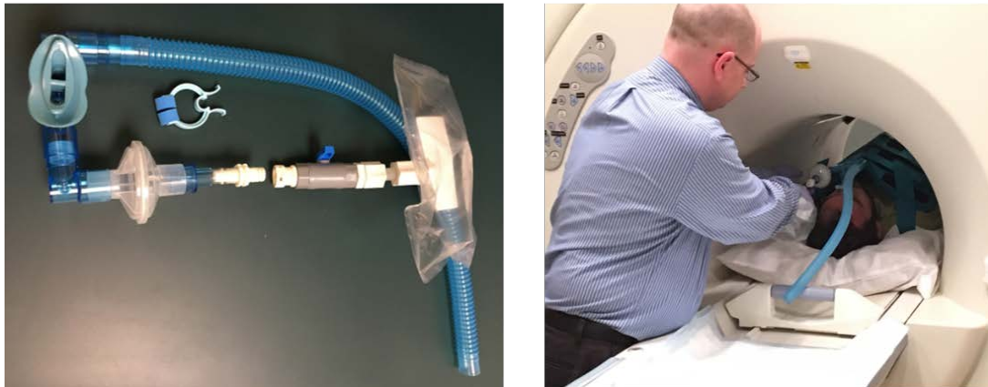
Figure 3.2. Example of home-made gas delivery apparatus (left) in use with the author pictured in MRI bore (right). Photo credit: Jeffrey Kammerman.
