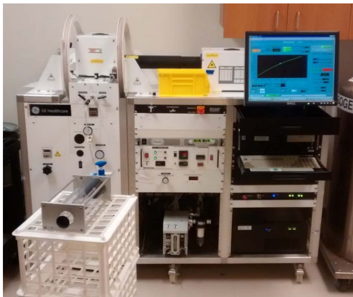
Figure 3.1. The primary helium hyperpolarizer used in the studies in this work (Polarean model IGI.9600).
