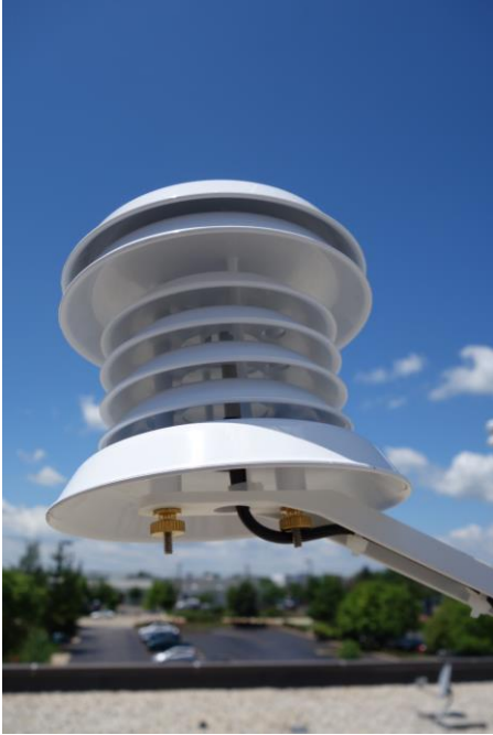
Photo 10-1 A close up view of a naturally aspirated solar radiation shield in place over an air temperature probe.
