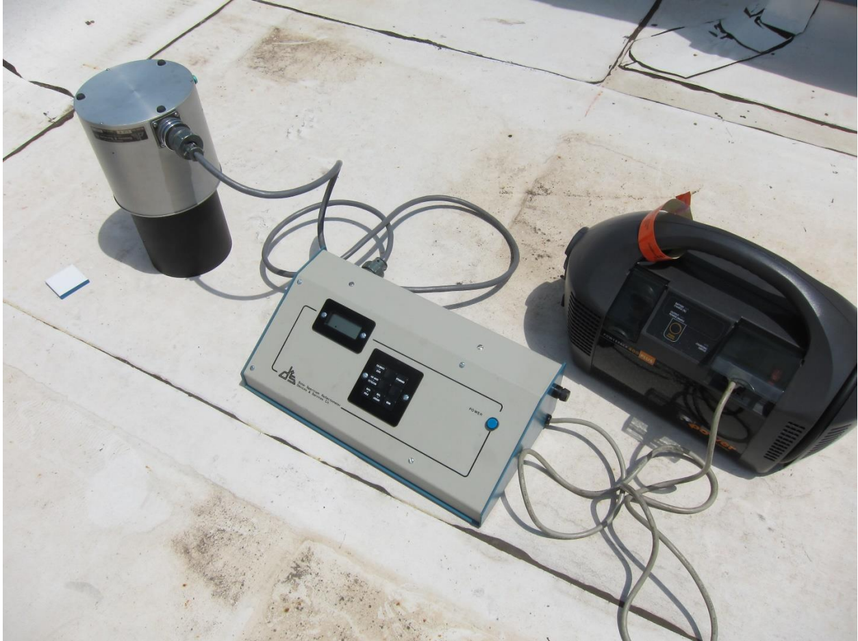
Photo 5-1 A SSR reflectometer in use during a 2012 study of field reflectivity in Texas.
