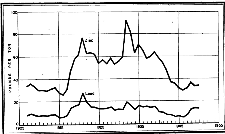
FIGURE 4.—Metal recovered per ton of crude ore (rock) milled in the Tri-State district, 1907-50.
