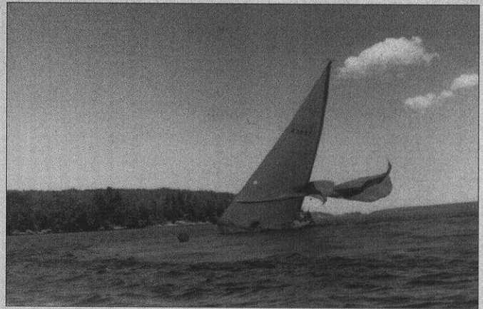
A competing boat displays what can happen if a spinnaker is not properly rigged.
