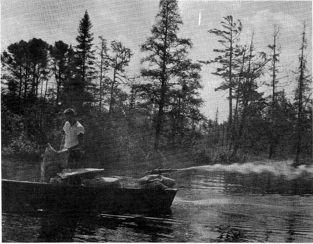
Fig. 20. Fritz Hasler, A. D. Hasler's son, sprays fluidized \text{Ca}(\text{OH})_2 hydrated lime or calcium hydroxide on Peter Lake to alkalize the water and precipitate the bog colloids that reduce water clarity, about 1952. The adjoining Paul Lake serves as the untreated reference lake. Peter and Paul Lakes are in the University of Notre Dame Environmental Research Center in Michigan. Source: Arthur Hasler.
