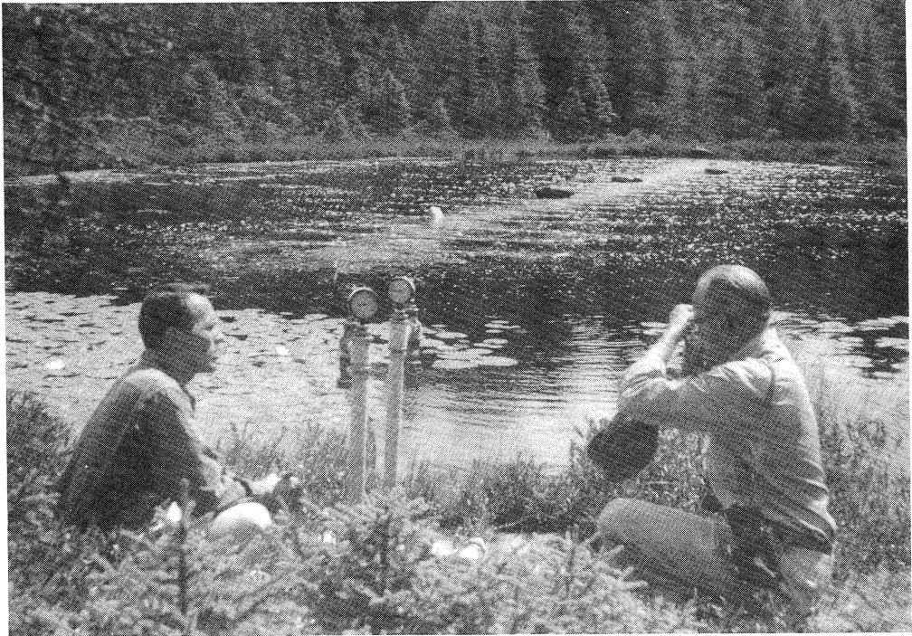
Fig. 21. William R. Schmitz and A. D. Hasler at Saw Mill Pond on the Guido Rahr Property adjacent to the University of Notre Dame Environmental Research Center, about 1956. They are studying the possibility of using air bubbles to "turn over a lake," that is, disturb the stratification of the lake and thereby aerate it. The air tube goes the full length of the lake. Source: Arthur Hasler.
