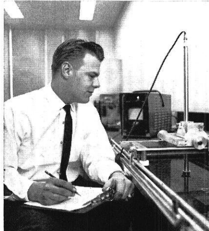
WALT BANTZ, E.E., SCRANTON '63 —Engineer at our research laboratories in Bethlehem, Pa., Walt is shown evaluating performance of ultrasonic equipment for detection of flaws in steel plates.
