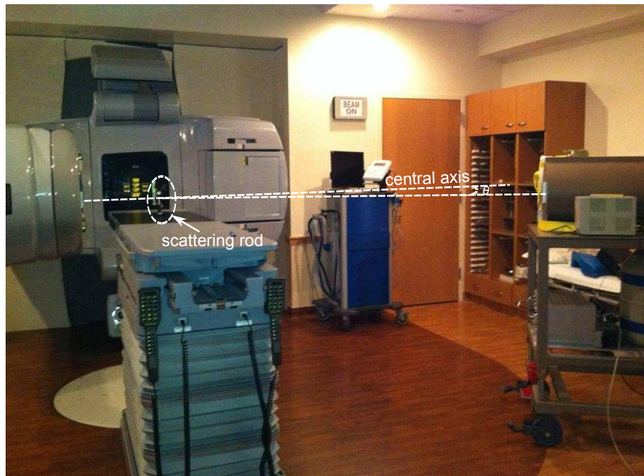
Figure 7.8: Photograph of the CS spectrometry system that was used for spectra measurements of the 6 MV beam from the Varian Clinac iX.
