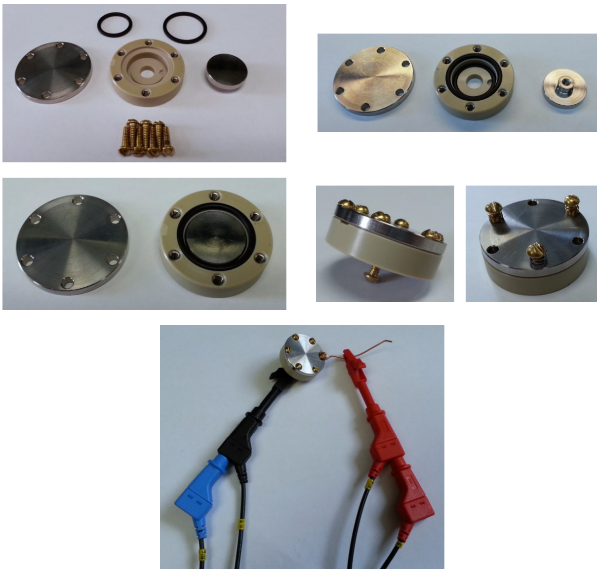
Figure A4.3. Images of cell used to measure conductivity of crosslinked gels. (top left) unassembled components including PEEK housing, Kalrez O-rings, stainless steel top and bottom electrodes, and brass bolts; (top right) cell with O-rings in place; (middle left) cell with bottom electrode in place; (middle center) fully assembled cell; (middle right) adapted cell for variable temperature EIS allowing motion of top electrode; (bottom) cell connected to potentiostat leads.
