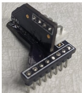
Fig. 4.1-2: Fabricated 3-D GMR PFD PCB (pictures taken at different angle)
