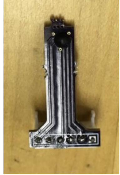
TMR PCB with potting and connector
