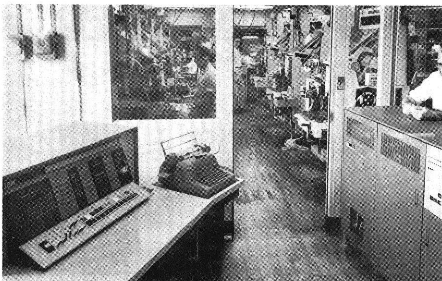
Figure 4.—COMPUTER—Shown at left is the IBM 1620 Computer. In the composing room are the Intertype Monarch Linecasters, at the right is the IBM Model II Buffer. (Courtesy South Bend Tribune )
