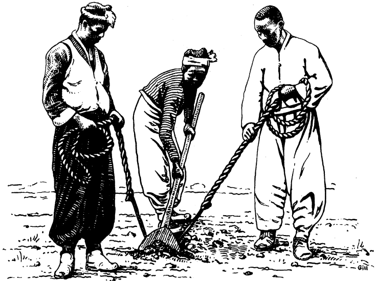
FIG. 78. Korean three-man spade, still occasionally used in remote parts of the peninsula
