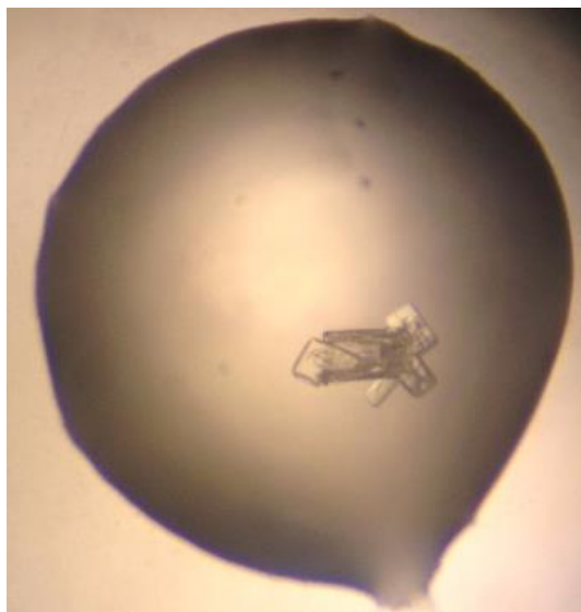
Figure A.21. Potential crystallization hit for EGFR-TM-F (Hampton research crystal screen II #47; crystallization conditions: DFK9008). Hanging drop vapor diffusion 2% w/v \beta -D-octyl glucoside. Crystal dissolved when pulled from the drop and mounted at room temperature in a mitogen sleeve.
