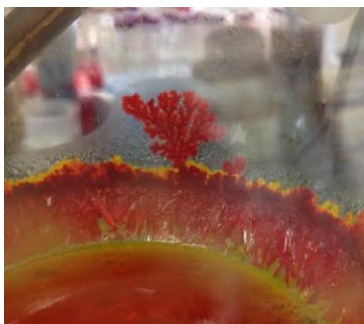
Figure B.18. Recrystallized DDQ deposited on the side of a round-bottom flask under vacuum.
