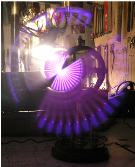
FIGURE 7: Geissler tube rotator in operation. Image from: http://www.earlytech.com/shop/view_item/1248700044
