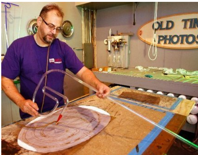
FIGURE 2: Neon sign bender Todd Paden at work in New Orleans, Louisiana, 2011. Note the presence of the pattern template below the tube. Image from: http://www.yelp.com/biz_photos/turks-inn-the-hayward?select=juhst4lqaHS3o_Gu5DE_9g#juhst4lqaHS3o_Gu5DE_9g
