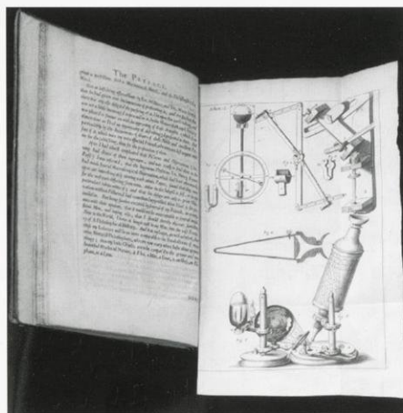
Fig. 9. Robert Hooke, Instrumentation including Wheel Barometer and Optical Microscope with Light Source, engraving, 14 \frac{1}{8} x 8 \frac{3}{4} in. Micrographia (London: The Royal Society, 1665) was one of the first publications of The Royal Society and one of the most important works in the history of science. Hooke invented the wheel barometer (depicted here) and made his microscopic observations through an instrument like that shown.
