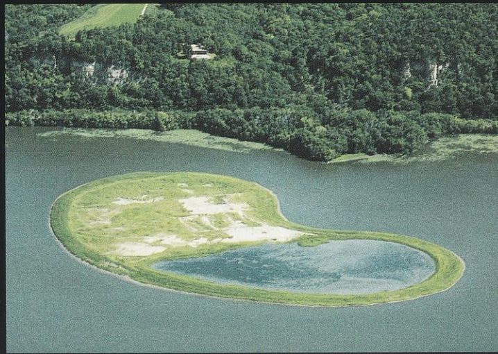
Sediment dredged from the channel project was formed into a 22-acre island that breaks up waves, and provides food and shelter for birds and turtles.
