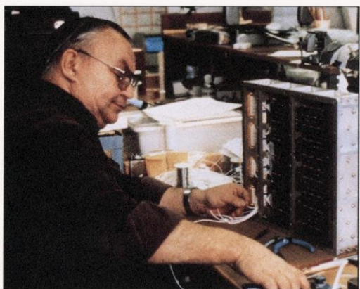
Gene Buchholtz assembles a detector controller for the Diffuse X-ray Spectrometer experiment.
