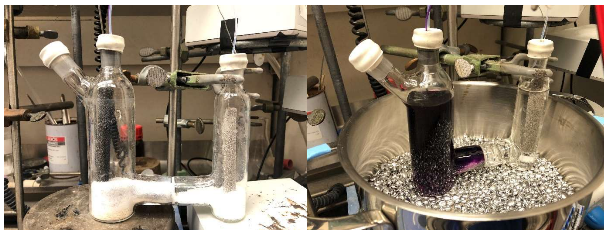
Figure E4. Left: Large scale divided cell batch assembly prior to addition of solvent. Right: Large scale divided cell batch assembly 5 minutes into electrolysis.
