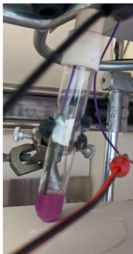
Figure F1. Undivided cell with submerged RVC and Ni foam electrodes.
