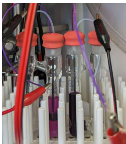
Figure F3. Divided cell electrolysis for dicationic adducts studies.
