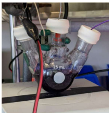
Figure F2. Undivided cell set-up for gaseous electrolysis.
