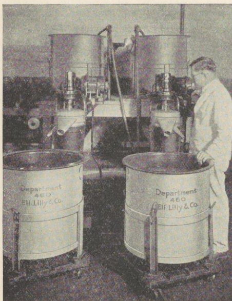
Tanks of extracted alcoholic liquid awaiting clarification by centrifuge.
