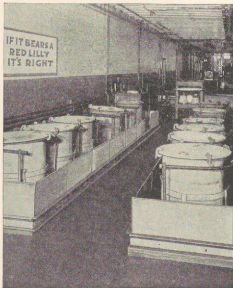
The clarification of the alcoholic extract by centrifuge.
