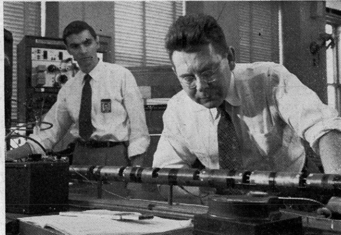
RELAYS VOICES UNDER THE SEAS. This is one of the repeater units in the new underseas telephone cables. These voice boosters make it possible for you to telephone Great Britain and Hawaii as clearly as you call across town. Developed by Bell Telephone Laboratories after many years of research. Made to entirely new precision limits by Western Electric.
