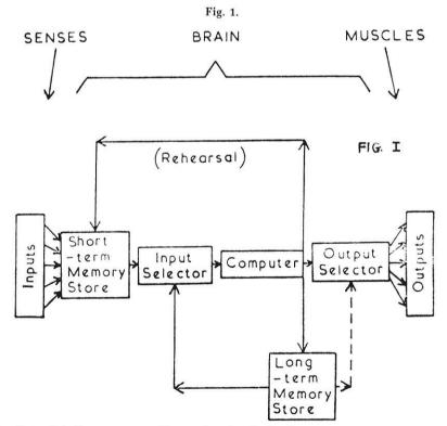
A simple model of man as a car dirver, showing the bottleneck in the brain through which all information has to pass if it is to be acted upon. The box labelled "Computer" works relatively slowly, unlike an electronic computer (Modified from Broadbent, 1958).
