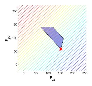
Figure 7.6: Feasible space of power generation for OPF problem 1 (Linear cost)
