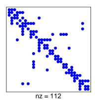
Figure 6.2: IEEE 30-bus system, Bus susceptance matrix *B*
