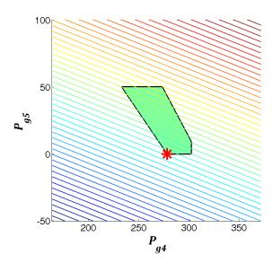
Figure 7.7: Feasible space of power generation for OPF problem 2 (Linear cost)
