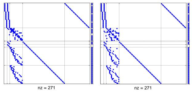
Figure 7.12: *M* matrix and *b* vector for OPF problem 1 (Piecewise-linear)
