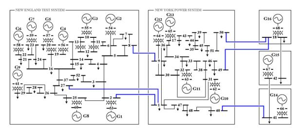
Figure 3.2: New England/ New York 16-machine 68-bus test system
