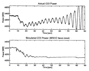
Figure 1.1: Actual vs. Simulated COI power flow, Aug. 10, 1996
