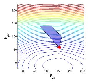
Figure 7.14: Feasible space of power generation for OPF problem 1 (Piecewise-linear)
