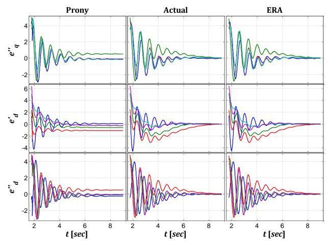
Figure 2.7: Simulated and estimated state variables  $e^{\prime\prime}_{\ q},\,e^{\prime}_{\ d}$  and  $e^{\prime\prime}_{\ d}$
