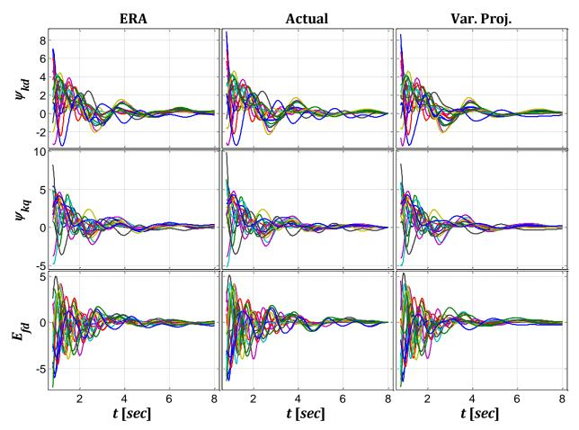
Figure 3.8: Simulated and estimated state variables  $\Psi_{kd}, \Psi_{kq}$  and  $E_{fd}$
