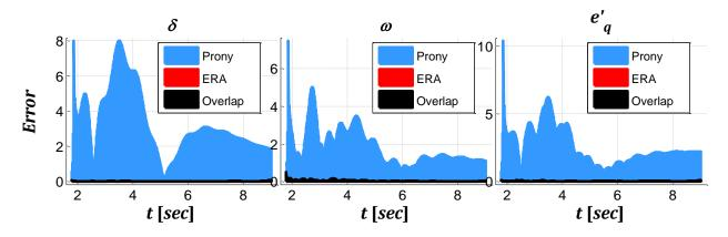
Figure 2.6: Estimation error for state variables  $\delta, \omega$  and  $e'_{\ q}$
