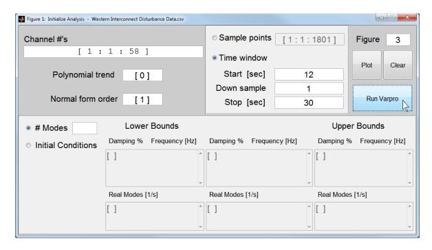
Figure 5.2: GUI for initializing modal analysis
