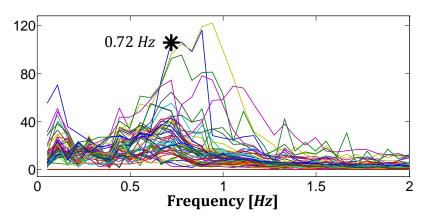
Figure 5.5: FFT of weighted residual error with 6 modes
