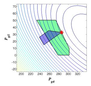
Figure 7.11: Feasible space of power generation for both OPF problems in coordinates of OPF problem 2 (Linear cost)
