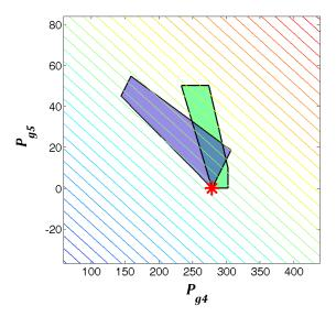
Figure 7.8: Feasible space of power generation for both OPF problems in coordinates of OPF problem 2 (Linear cost)
