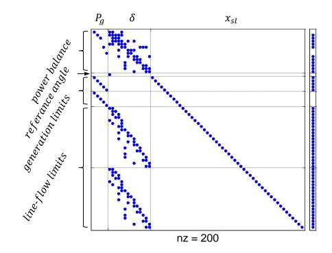
Figure 7.1: *M* matrix and *b* vector for IEEE 14-bus system
