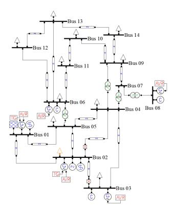
Figure 2.4: IEEE 14-bus Simulink Model
