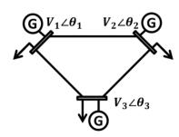
Figure 4.1: Three-bus power system
