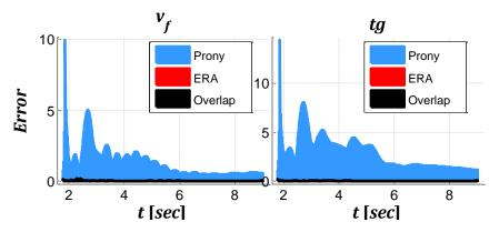
Figure 2.12: Estimation error for state variable  $v_f$  and turbine governor state variables
