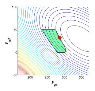
Figure 7.10: Feasible space of power generation for OPF problem 2 (Quadratic cost)
