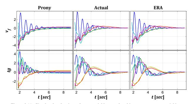
Figure 2.11: Simulated and estimated state variable  $v_f$  and turbine governor state variables
