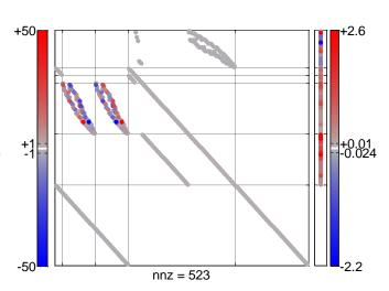
Figure 6.5: Nonzero elements of  $P_1M'$  in 30-bus system
