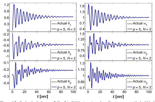
Figure 4.5: Optimal solution p = 5, N = 2 (solid blue) vs. Actual nonlinear response (dashed black)
