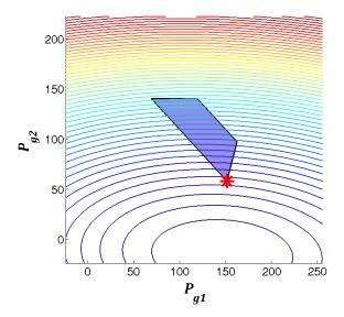
Figure 7.9: Feasible space of power generation for OPF problem 1 (Quadratic cost)
