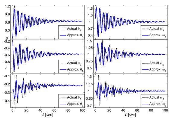
Figure 4.2: Linearization solution (solid blue) vs. Actual nonlinear response (dashed black)
