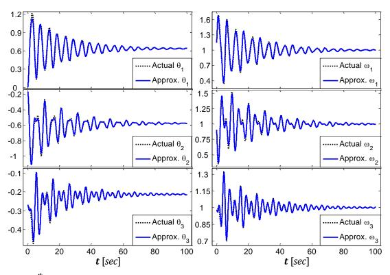
Figure 4.3: 8<sup>th</sup> order normal form solution (solid blue) vs. Actual nonlinear response (dashed black)
