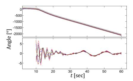
Figure 3.1: Bus angle disturbance data (a) without trending removed (b) with trending removed
