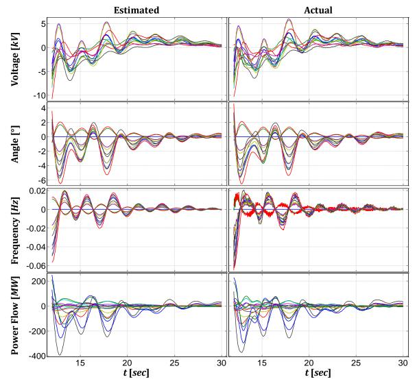
Figure 5.4: Estimated solution with 6 modes vs. Actual data
