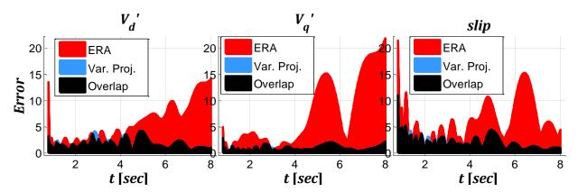
Figure 3.11: Estimation error for state variables  $V^{\prime}_{d}, V^{\prime}_{q}$  and slip
