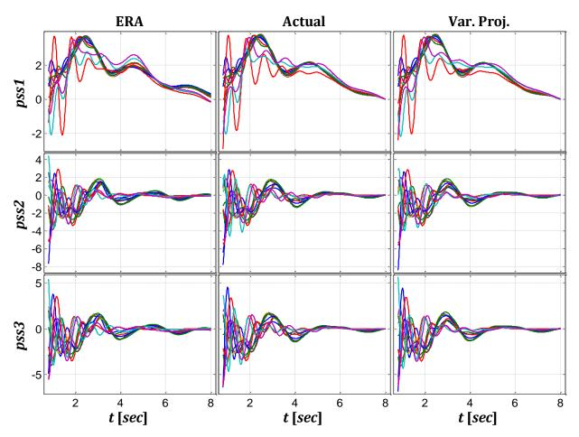
Figure 3.12: Simulated and estimated state variables pss1, pss2 and pss3
