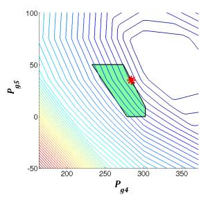
Figure 7.15: Feasible space of power generation for OPF problem 2 (Piecewise-linear)
