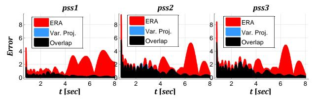
Figure 3.13: Estimation error for state variables pss1, pss2 and pss3
