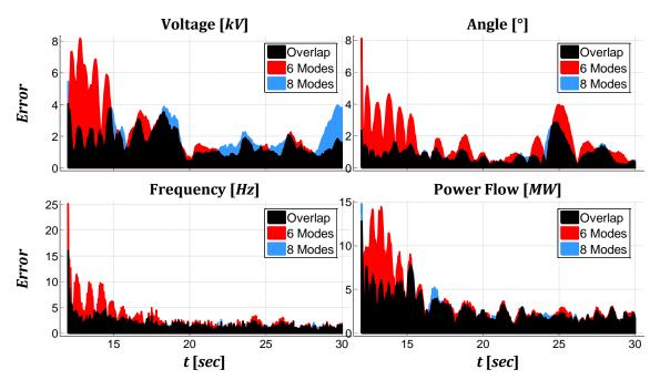
Figure 5.8: Weighted residual error comparison for 6 modes vs. 8 modes
