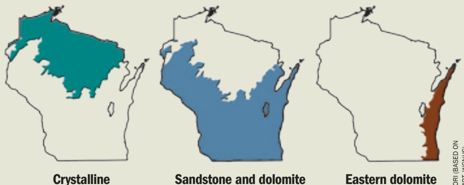
These maps show the location of three types of bedrock aquifers in Wisconsin. A fourth, the sand and gravel aquifer, is the sediment covering most of the state except parts of the southwest.
