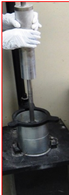
6. Compaction in the Marshall Hammer
