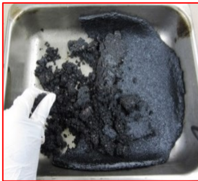
5. Break Mixture While at 60°C
