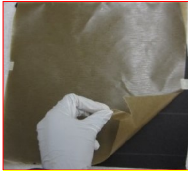
1. Apply Non-stick Paper to Felt
