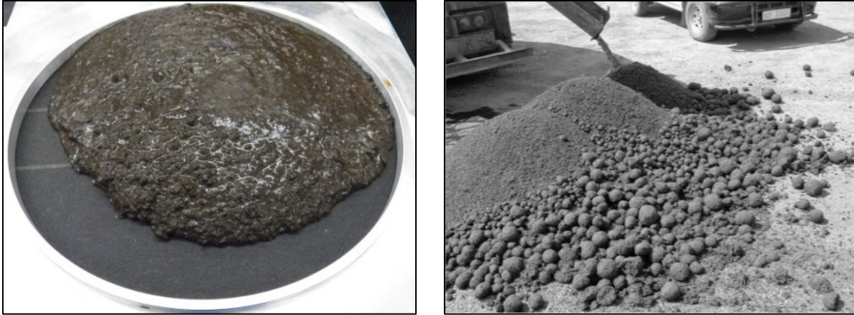
Figure 3. Example of a slurry or micro-surface with sufficient mix time (left) and on with insufficient mixing time (right) (SABITA, 2012)
