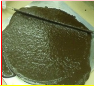
2. Cast Mixture in WTAT Molds
