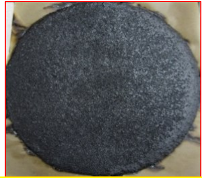
3. Cure in Oven for 24hrs@ 60°C
