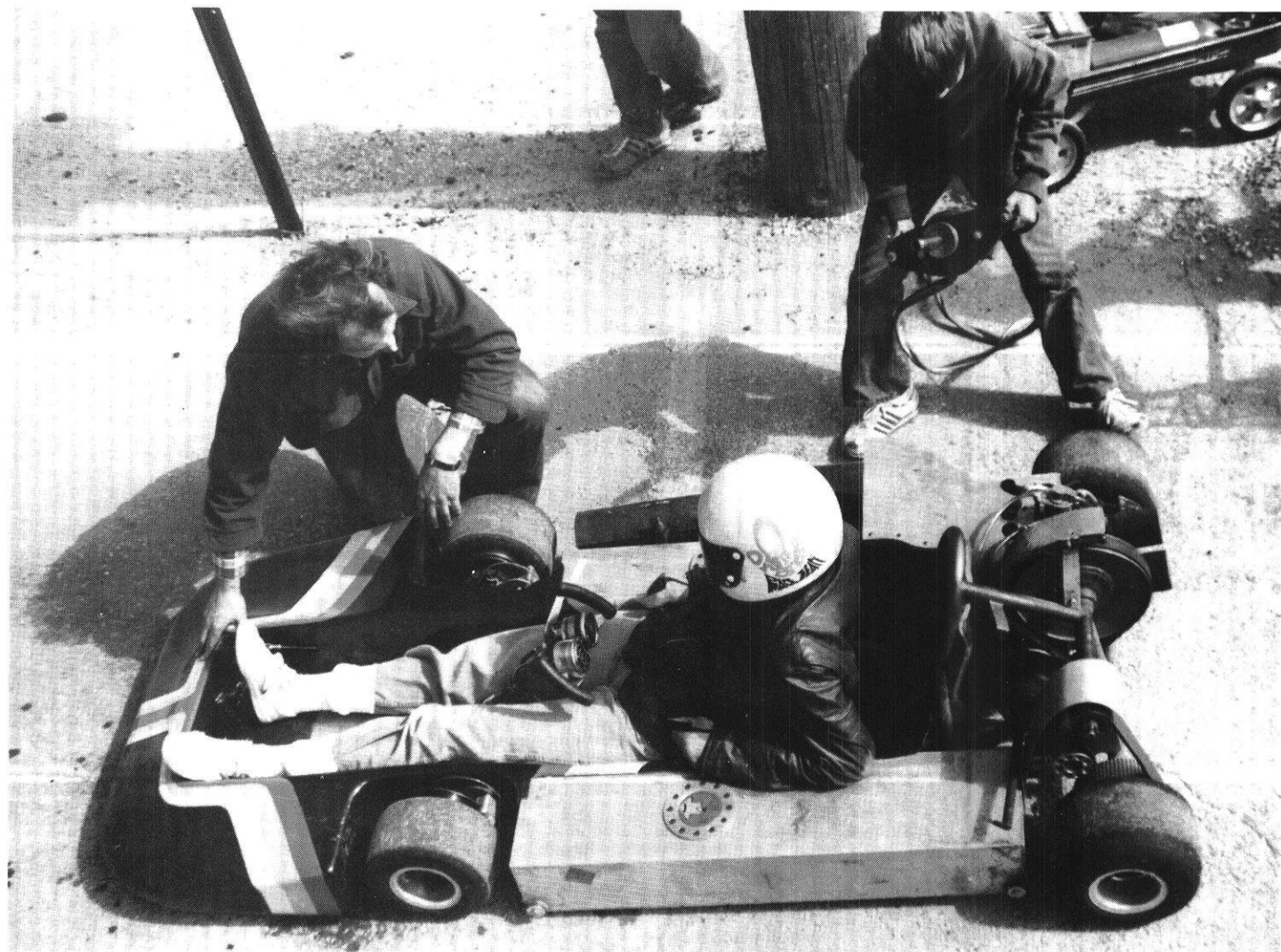
An unusual entry to the race, this go-cart receives a start from a separate electric starter.
