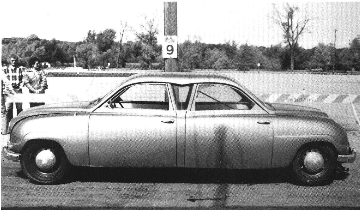
Is it coming or going? This hybrid experimental car is comprised of the front sections of two Saabs welded together. Not ideally suited to racing, it received the slowest time of the day.
