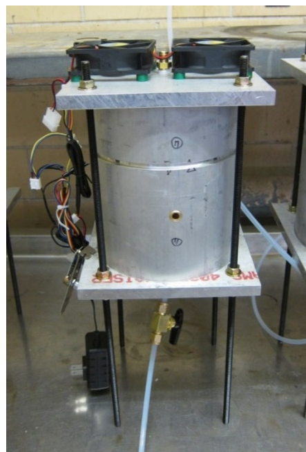
(b) Magnetic stirrer with switch and electrical adaptor and setting up on top plate of testing column
