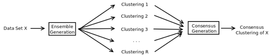
Figure 4.1: Ensemble Clustering. The typical flowchart of an ensemble clustering framework. Multiple clusterings of a single data set X are generated by varying parameters, perturbing the data, and subsampling. The collection of these clusterings, called an “ensemble” is then input to a consensus step that attempts to combine information from all these clusterings and generate a final consensus clustering from them.
