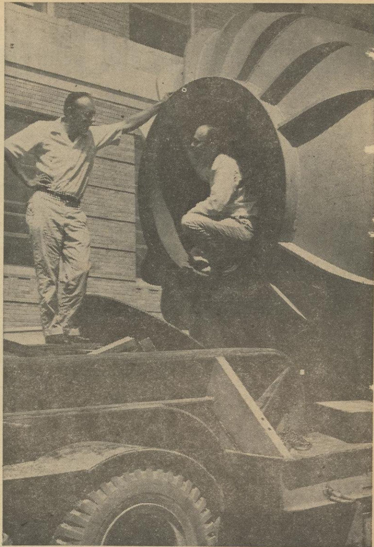
TUBE —Shown ushering in the 23-ton steel tube which is the vacuum tank of the atom smasher, is Willy Haeberli (left) and Hugh T. Richards of the Physics Dept. The machine arrived at the University in 1959.
