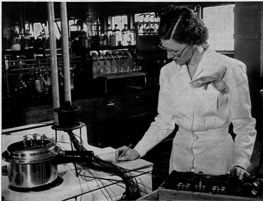
TAKEN IN the department's research lab in experimental foods, this picture shows the apparatus used in experiments on rate of heat penetration as related to destruction of food poisoning bacteria. The problem is being tackled by Maxine McDivitt, a Ph.D. candidate, shown checking data.
