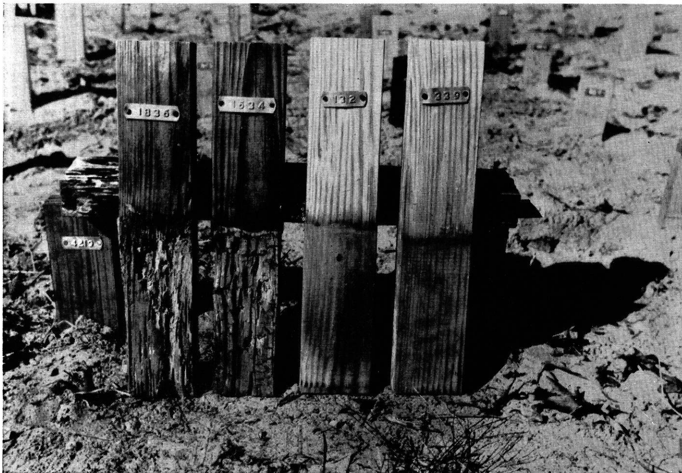
Wood specimens which show the excellent preservative qualities of Pentachlorophenol. The two pieces on the right were impregnated with this protection against decay. All four pieces were buried underground for six years in a Dow test plot.
