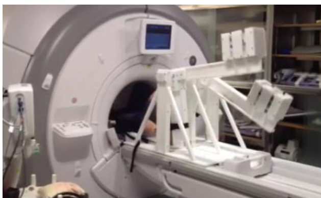
Figure 4-2: Low-cost MR-compatible stepper developed at the University of Wisconsin-Madison. Subjects exercise via a dynamic stepping motion in a supine position in the MRI bore. Resistance is determined by removable weights included in the boxes at the end of each lever arm.
