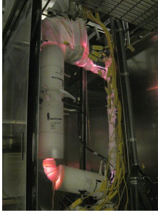
Figure 6: Photograph of a thermal convection corrosion loop constructed with Hastelloy N (courtesy ORNL).
