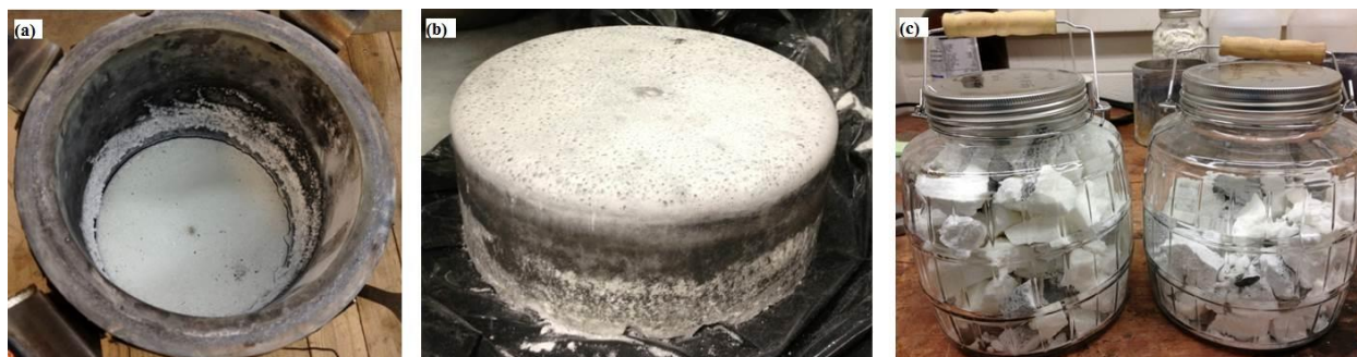
Figure 16: Salt prepared at the University of Wisconsin laboratory: (a) Laboratory made 20kg KF-ZrF 4 in SiC-coated tank, (b) bulk salt and (c) salt chunks stored in glass jars.
