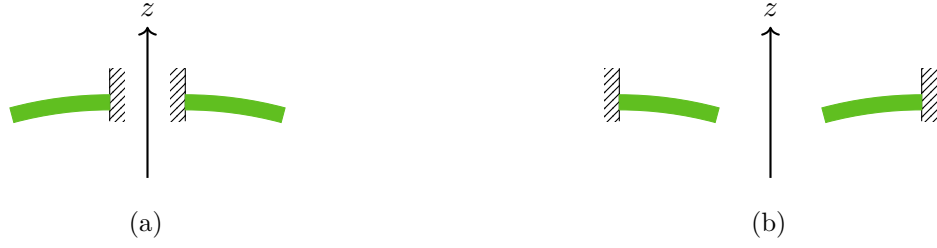
Figure 6.13: Annular plate with a uniformly distributed pressure p over the entire plate [107] (a) rotor plate: outer edge free, inner edge fixed (b) stator plate: outer edge fixed, inner edge free.
