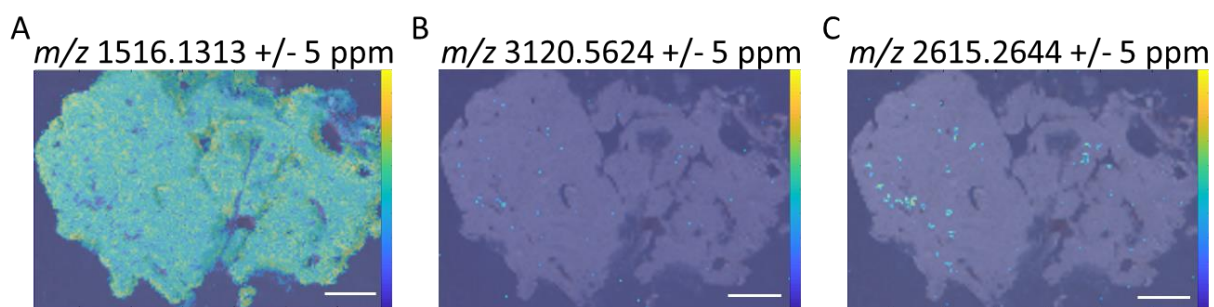
Figure 1. Three example MALDI-MSI images acquired on the MALDI-Orbitrap with DHB as the matrix. The white scale bar indicates 2 mm.
