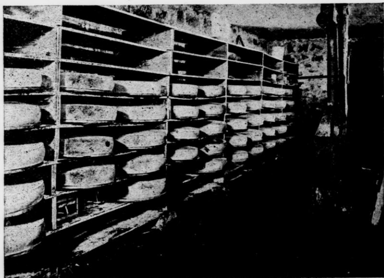
FIG. 9.—Curing cellar in Five Corners factory, near Monroe. The large drum Swiss cheeses are on the shelves. The small boiler supplies steam for moisture when too dry.
