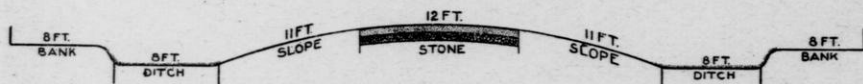
Section of permanent country road, with 12 ft. stone track and sloping shallow ditches for sled track in winter, when needed.
